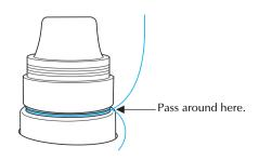
Pass the thread along the thread path indicated on the machine, and then pass it under the number 1 middle thread guide plate.
